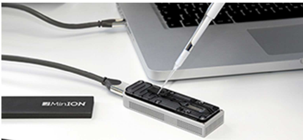
Figure 3: The MinION: the first palm sized sequencer
