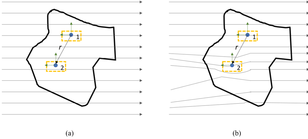
Figure 30: (a) two magnetometers sense the same local Earth’s magnetic field in absence of additional external fields. (b) in presence of disturbances, the two magnetometers sense two different local magnetic fields due to their relative distance r . Figure taken from (Caruso, Sabatini, Knaflitz, Gazzoni, et al., 2021).
