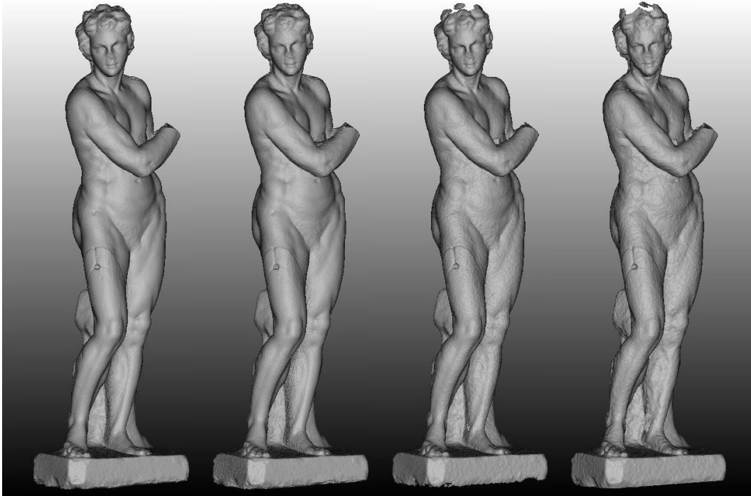
Figure 5.32 Photogrammetric models, statue from the Fountain of Hercules (from left to right): AMP VIS, AMP NIR, FZA VIS, FZA NIR
