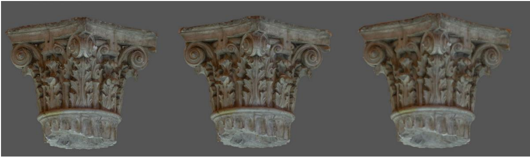
Figure 5.22. Textured photogrammetric meshes of the capital replica from dataset 5, (from left to right) AMP, VCM, R3D.
