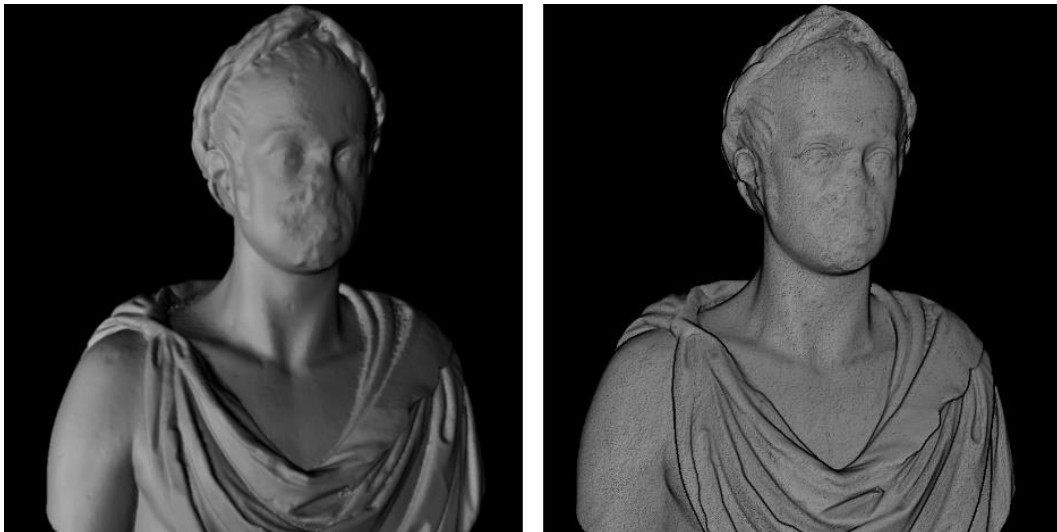
Figure 4.37. Visualizations of digital model in CloudCompare with approximated normal rendering using SSAO shader (left) and Sobel filter-based solution (right).
