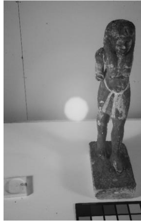
Near infrared reflectance image, Nikon D810 + Hoya R72 filter
