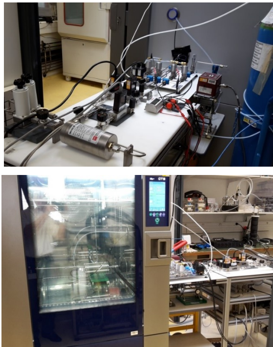
Figure 11. Overview of facility, from the left to the right, humid air generator, divider plate, climatic chamber with testing chamber
