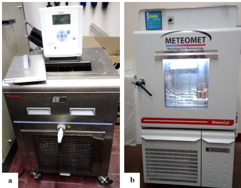
Fig. 10. Thermostatic bath (a) and climatic chamber (b) with inside the sensors in calibration, the reference sensor and copper comparing blocks
