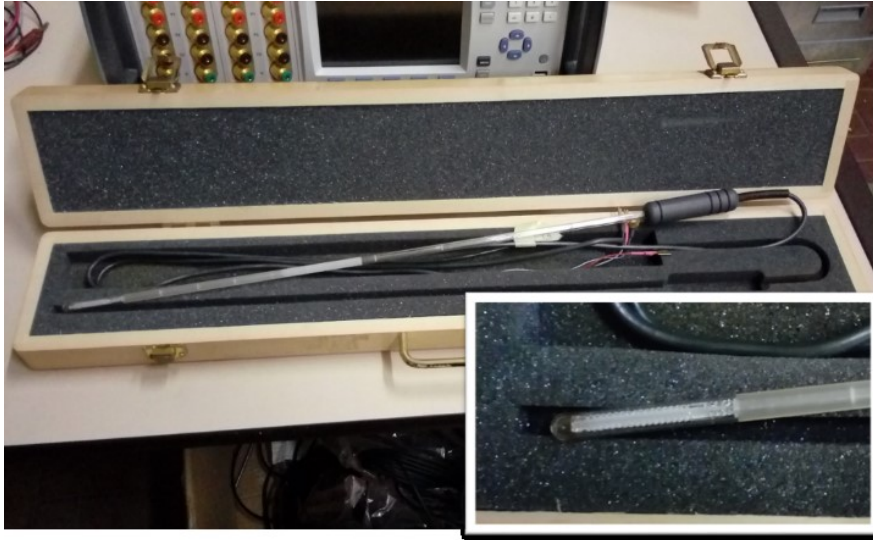
Fig. 11. Quartz sheath, long stemmed Capsule Standard PRT (C-SPRT) 25 \Omega , reference standard used in primary laboratories and particular of the sensing element
