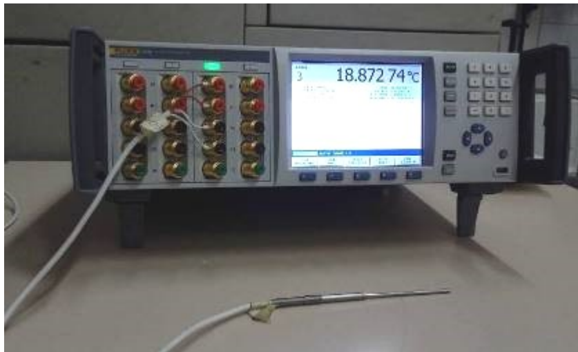
Fig. 9. A Pt100 secondary reference standard connected to a resistance measuring bridge of high accuracy
