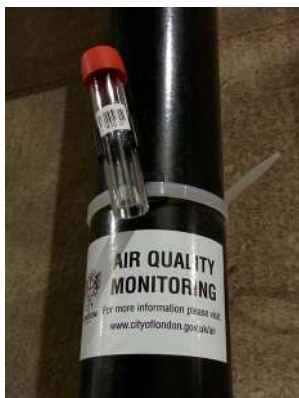
Figure 6. A typical diffusion tube attached, by a cable tie, to a drainpipe. The bottom end is open to the atmosphere. Pollution is captured by a chemical inside the red cap at the top 69 .
