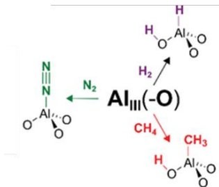
Figure 52. Schematic representation of the adsorption of \text{N}_2 and of the splitting of \text{CH}_4 and \text{H}_2 on \text{Al}_{\text{III}} defective sites. Adapted from ref. 59
