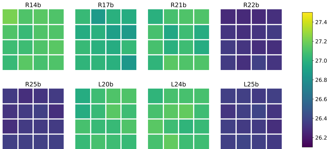
Figure 4.46: Breakdown voltage distributions at 20 °C for the SiPM arrays under study
