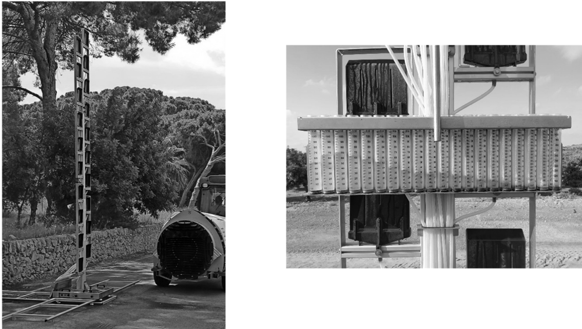
Figure 6. Vertical spray profile distribution evaluation system (left). Cylinders where the spray collected by height accumulates (right).
