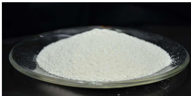
Figure 9. Pictures of the oxide powder obtained as a result of the synthesis process (in this case: \text{CeZn1-NO}_3 )
