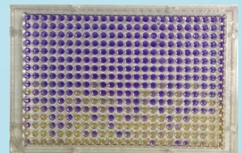
Ames test in 384-wells plate
