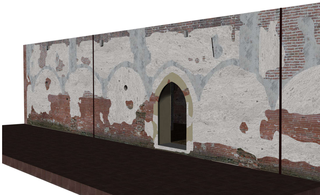
Figure 188. Texturized rendered NURBS model of the refectory. South front of the cloister, detail on stratigraphic units (elaboration F. Diara).
