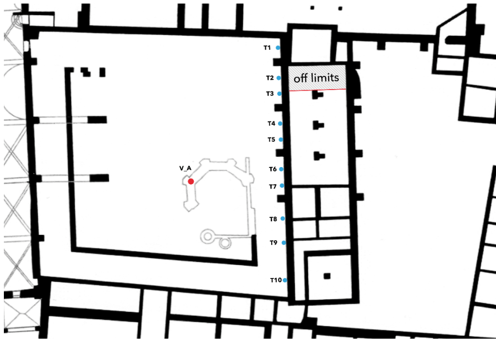
Figure 59. Topographic survey: targets from T1 to T10 on the south front of the cloister
