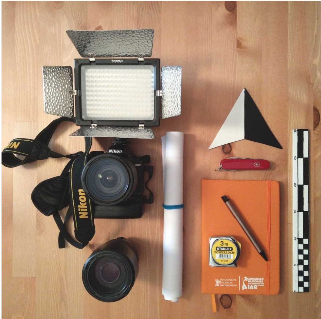
Figure 42. Base equipment for a stratigraphic survey: camera, meter and notebook are fundamental
