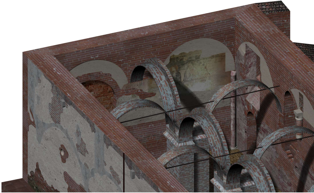
Figure 195. Texturized rendered NURBS model of the refectory. Internal detail of the east wall and arches (isometric view) - (elaboration F. Diara).
