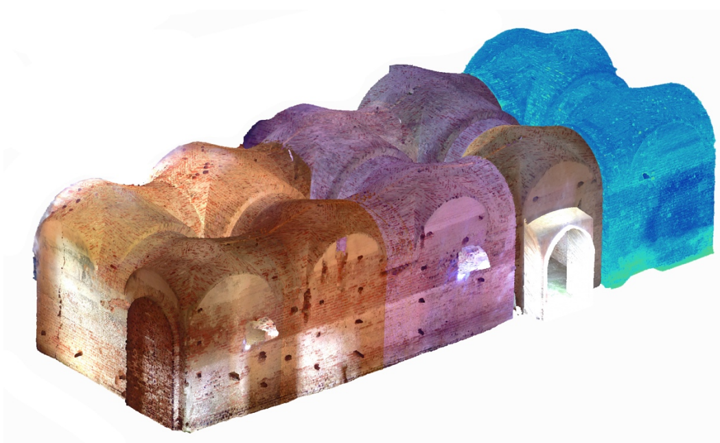
Figure 84. Cleaned point clouds related to the whole refectory (perspective view) - (elaboration F. Diara).
