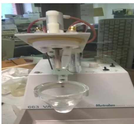
Figura 1. Electrolytic cell in a conventional voltammetric analyzer.
