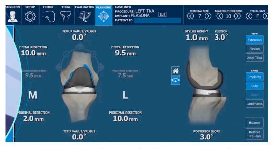
**Figure 7.** Intra-operative phase with summary of implant positioning, amount of resection, and alignment evaluation.
