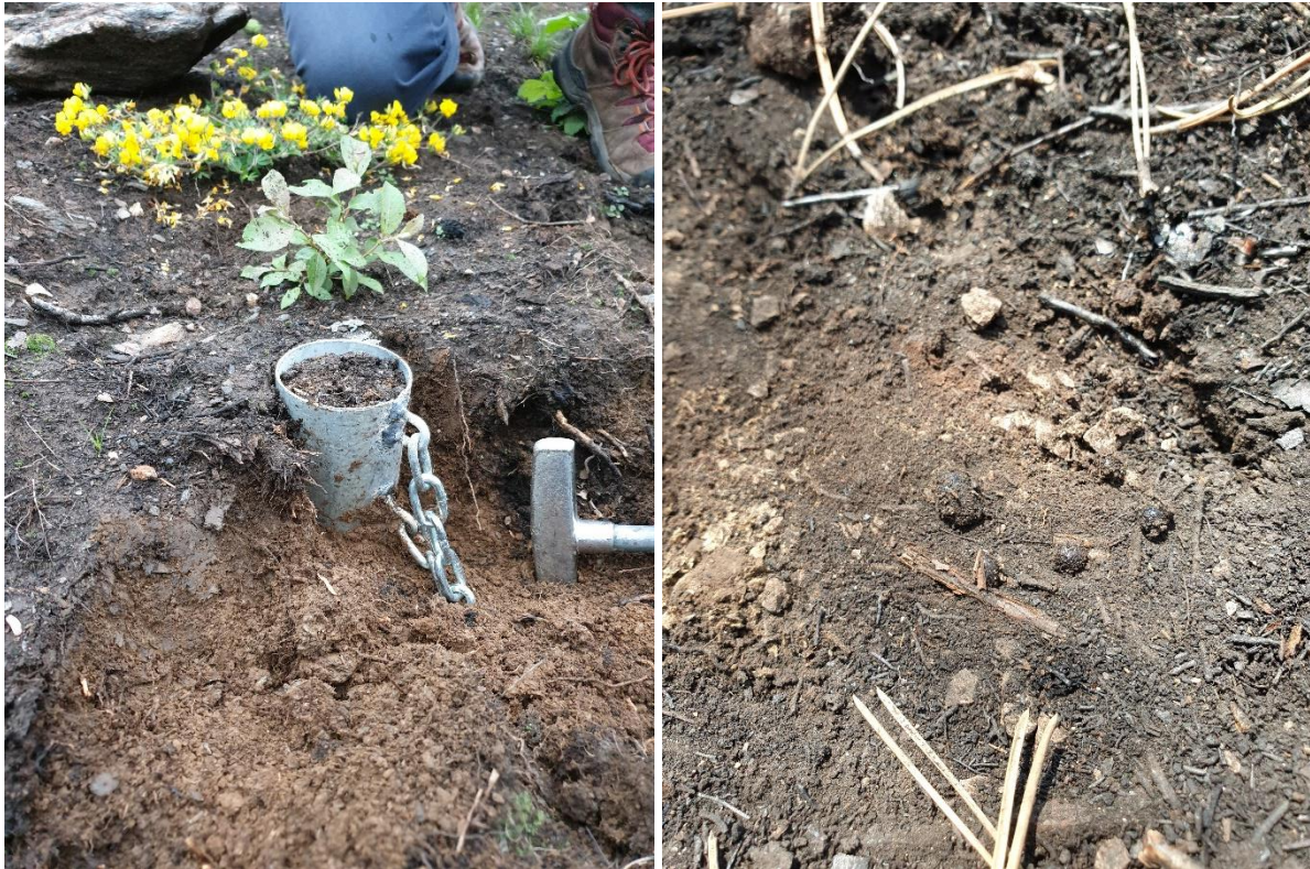
Figure 7.6 - empirical shear tests device (left) and Water Drop Penetration Time test for hydrophobicity assessment (right).
