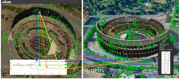
Figure 2. Implementation of historical deformation analysis of the Flavian Amphitheatre, Colosseum Archaeological Park, Italy, whose geometric and material characteristics made it particularly suitable for structural monitoring with interferometric processing and analysis (COSMO-SkyMed data processed by e-GEOS) (reproduced from Della Giovampaola, 2021).
