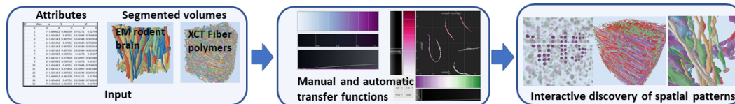
Figure 1: Inspired by word search puzzles, we present Volume Puzzle , a framework that allows us to interactively and/or automatically reveal spatial patterns from segmented volumes with associated multivariate attributes
