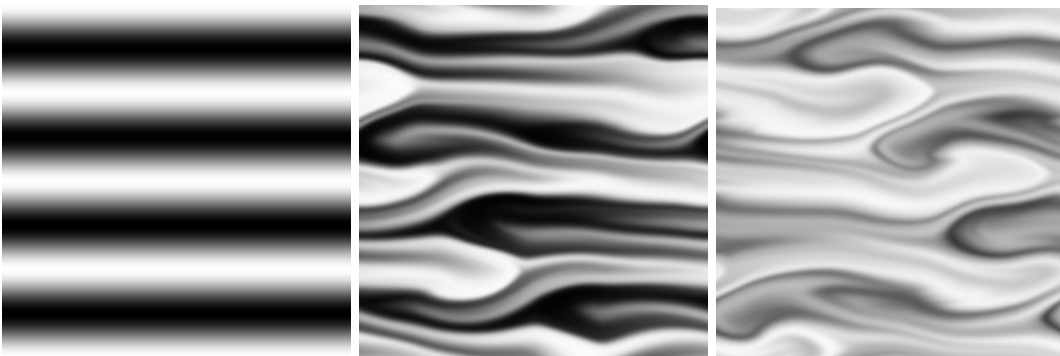
FIG. 9: Vertical section in the x - z plane at fixed y = 0 of the scalar field \theta for the 3D simulation with \eta = 8 at different times. From left to right: t = 0 , t = 32T_0 , t = 64T_0 .
