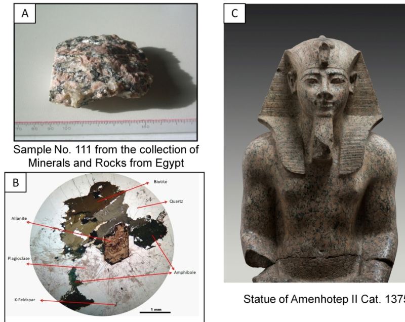
Fig. 3 - Monumental pink granite form. Macroscopic (A) and microscopic (B) image of Sample No. 111 from the collection of Minerals and Rocks from Egypt; C) Statue of Amenhotep II exposed at the Museo Egizio of Turin (cat. 1375).
