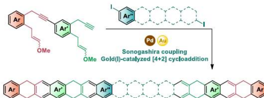
Figure 1. General synthesis of higher hydroacenes, starting from tridecacene-H8.
