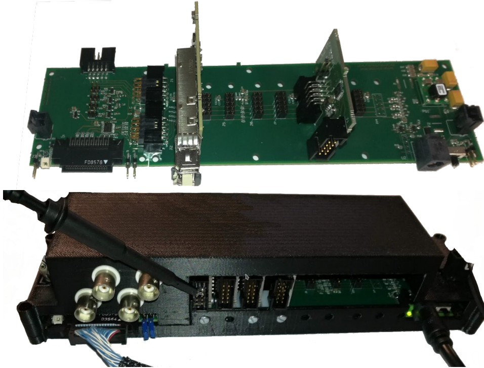
FIGURE 2.8: Local FCS Fanout module. The top picture shows the L-FCS-F PCB, with the modular slots for the connection of optical transceivers or LVDS connectors. The bottom picture shows the L-FCS-F enclosed in its 3D printed case.
