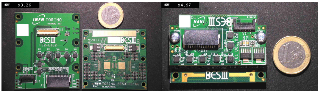
FIGURE 2.4: Picture of the FEBs. Left: the layer 1 and layer 2 design. Right: the layer 3, more compact, design.
