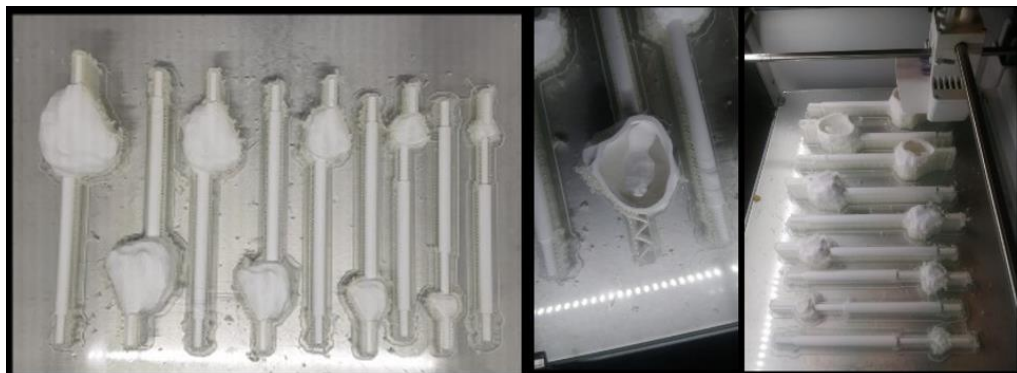
Figure 3.9 – First attempt of 3D printed inserts production with PLA material.
