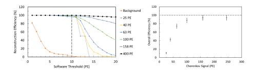
**Figure 6:** Left: Reconstruction efficiency of Cherenkov events compared to accidentals events (orange) for different photoelectron (PE) intensities. Right: Combined trigger and reconstruction efficiency of Cherenkov events as a function of the detected Cherenkov signal.
