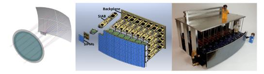
**Figure 2:** Left: Schmidt catadioptric optics of the Cherenkov telescope. The mirrors focus the light onto the curved focal plane located between the corrector plate and the mirror. Middle: CAD drawing of the camera without housing. Right: Half assembled camera (Lego figures for scale).
