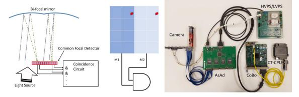
**Figure 3:** Left and Middle: The bi-focal optics duplicates the image and projects it to two separate locations in the camera. The telescope readout is triggered if two pixels separated by the bi-focal split record a signal within 100 ns. Right: Partially assembled camera and the readout electronics.
