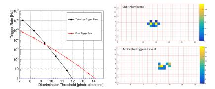
**Figure 5:** Left: Simulated trigger rates caused by background fluctuations for a single pixel in the camera and the 512-pixel camera after applying the bi-focal trigger. Right: Camera event display of a simulated air-shower event (top) and accidental-triggered event (bottom).
