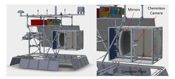
**Figure 1:** Left: EUSO-SPB2 payload, with the Fluorescence telescope pointing down for detecting UHECR and the Cherenkov telescope pointing at the Earth limb to detect VHE-neutrinos below-the-limb and UHECR via Cherenkov radiation above-the-limb. Right: Close-up of the Cherenkov telescope with the corrector plate.
