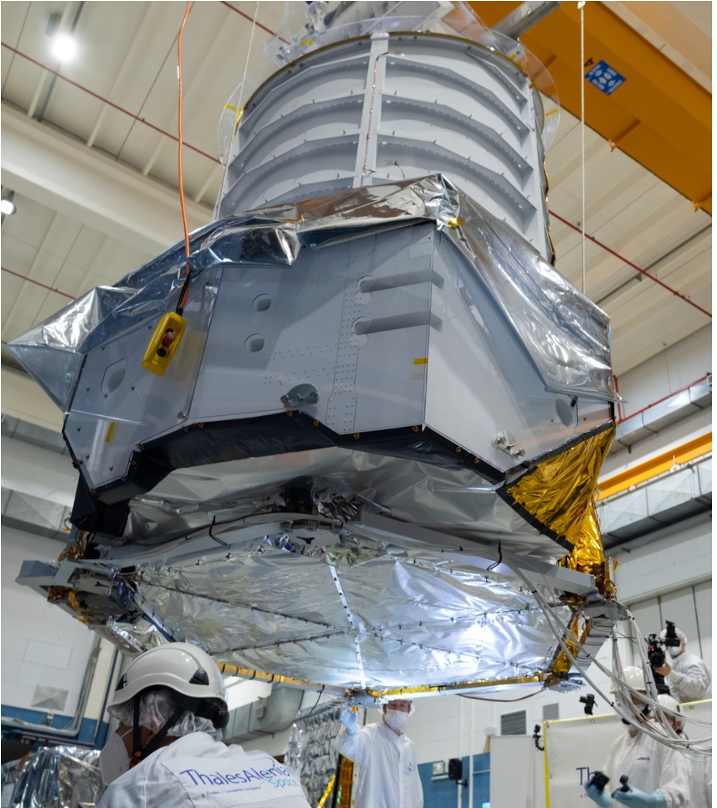
Fig. B.4. Bottom of the PLM, shortly before the mating with the SVM shown in Fig. B.3. The bottom is covered with MLI to provide thermal insulation and to prevent molecular contamination entering from the SVM. The large white polygonal structure girding the lower parts is the NISP radiator. A high-resolution image is available after account creation from the ESA Photo Library For Professionals at https://www.esa-photolibrary.com/ESA/media/65700 . The PLM was built by Airbus Defence and Space. Credit: ESA - S. Corvaja.
