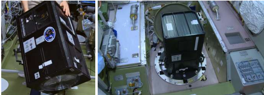
Fig. 9 Left: Mini-EUSO telescope managed by the cosmonaut before to be installed on the nadir-facing UV transparent window of the Zvezda module. Right: Mini-EUSO mounted on the UV transparent window. The velocity vector is usually toward the bottom of the picture, in the side marked as '1'.
