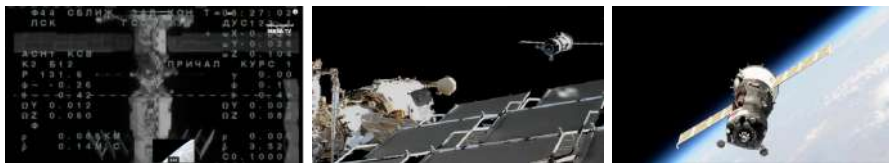
Fig. 8 Left: the first failed docking attempt on the Poisk module docking port, on 2019 August 24. Center: relocation of the Soyuz MS-13 capsule from the Zvezda module docking port to the Poisk module docking port. Right: second, successful, docking attempt on the Zvezda docking port, on 2019 August 27.
