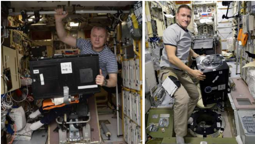
Fig. 11 Left: the cosmonaut Oleg Novitskiy with Mini-EUSO. On the bottom of the picture is visible the pouch with the data cards. Right: Cosmonaut Ivan Vagner with Mini-EUSO prior to its installation on the UV transparent Zvezda window (center bottom of the figure). The instrument front lens is visible between the hands of the cosmonaut.
