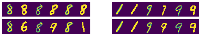
Fig. 7. Reconstruction: VAE (upper) vs. V-ABC (lower); MNIST data set ( p = 0.2 ). Original and reconstructed data are alternated. Threshold filter applied. The unwanted digit ‘8’ is reconstructed to the same digit only for the VAE.
