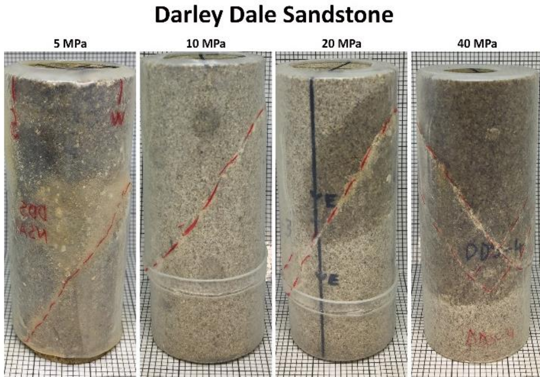
Figure 2.7: Post-experimentation imaging of Darley Dale Sandstone. Shear zone structure is highlighted in red.
