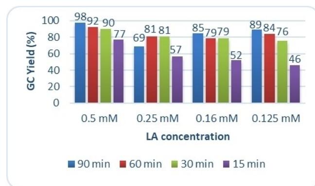
Figure 5. MW-assisted reductive amination of LA with p -anisidine using CPME as solvent: optimization of reaction time and LA concentration.
