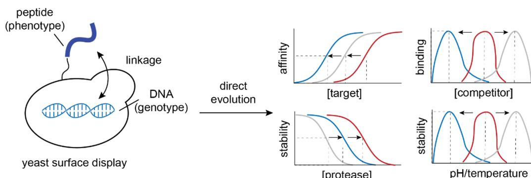
**Figure 1**, Schematic representation of yeast display technology that relies on a physical linkage between the display peptide sequence (phenotype) and its encoding DNA sequence (genotype). The yeast display platform via a direct evolution approach allows the selection and the engineering of key peptide properties, such as affinity, binding specificity, thermal and chemical stability.
