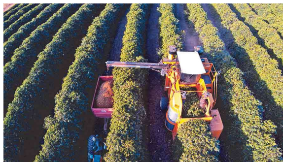
Figure 10. Coffee harvesting technique through machinery called "stripping".
