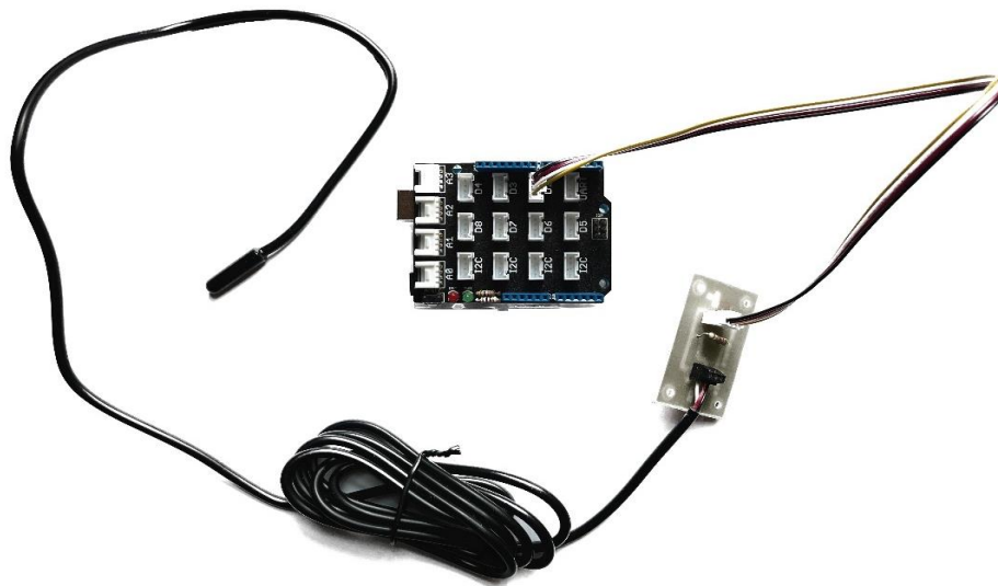
Figure 21 The body temperature sensor connected to the Arduino prototyping platform
