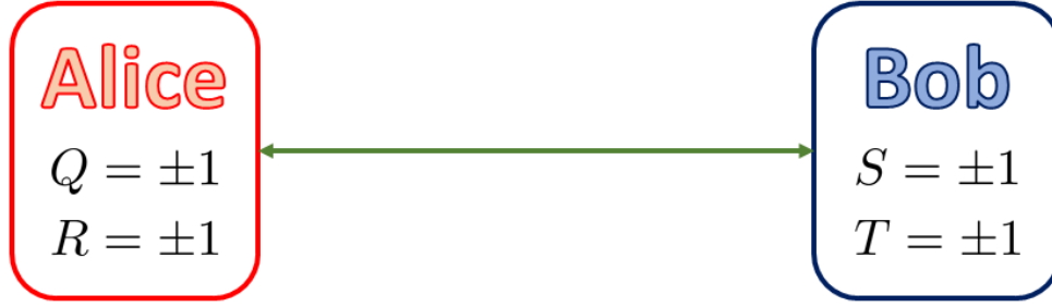
Figure 1.1: Schematic experimental setup for the Bell inequalities. Alice can choose to measure either Q or R , and Bob chooses to measure either S or T . They perform their measurements simultaneously. Alice and Bob are assumed to be space-like separated, i.e. far enough apart that performing a measurement on one system can not have any effect on the measurement results on the other.
