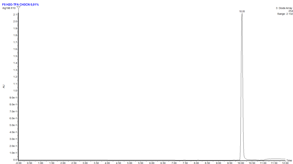
Figure S5.5: HPLC chromatogram revealed at 254nm of pure 5 .
