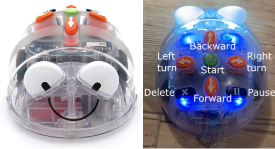
Figure 1. Blue Bot (front and above view) and the buttons with the commands on its back
