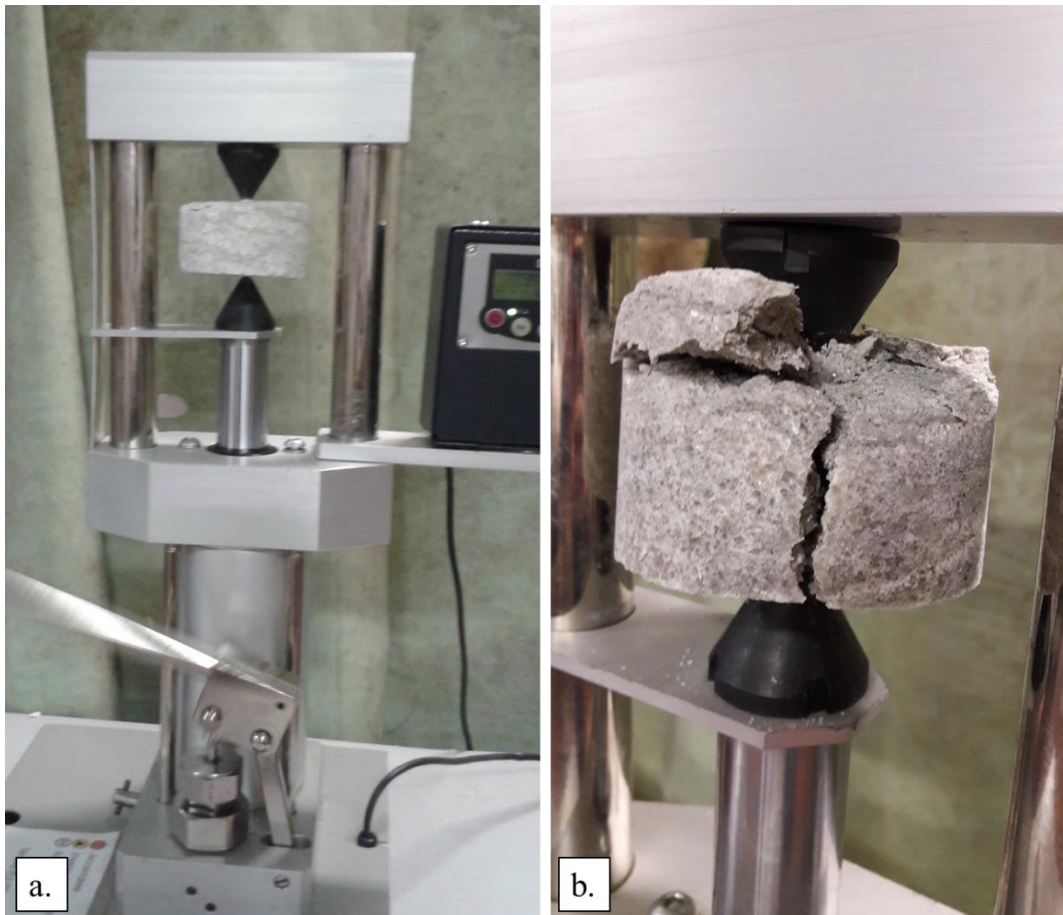
Figure 5.3 a. Point Load test equipment. b. Detail of sample failure under the application of the punctual load with the conical points
