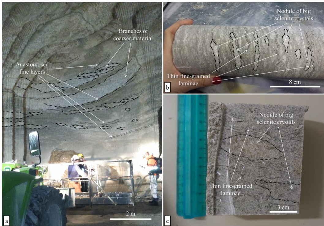
Figure 3.9 a. Excavation face in a gypsum underground quarry in Monferrato (NW Italy). It is evident the typical structure of the branching selenite gypsum, with branches of coarse material surrounded by anastomosed fine layers. b. Core sample of branching selenite gypsum, with nodules of coarser gypsum crystals surrounded by thin fine-grained laminae. c. Hand sample, with a more detailed scale, with nodules of coarse gypsum crystals surrounded by thin fine-grained laminae
