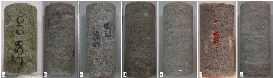
Figure 6.4 Cylindrical samples for the triaxial test (denominated with alphabetic letters from a to g)
