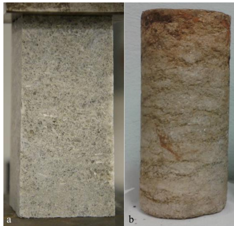
Figure 3.11 Macroscopic appearance of A-type (a) and B-type (b) gypsum samples
