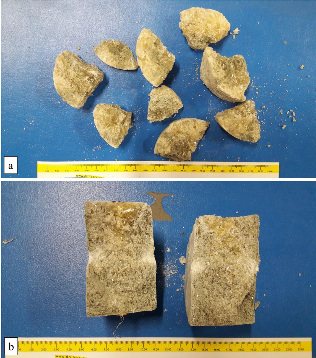
Figure 5.9 a. After-failure rock fragments of B-type samples. b. After-failure rock fragments of A-type samples.
