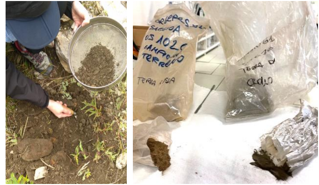
Fig. 3. Sampling Procedure and Soils Samples sieved 90\ \mu\text{m} .
