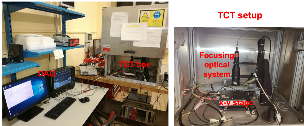
Figure 6.13: TCT setup in the laboratory of the Innovative Silicon Sensor, in Turin.
