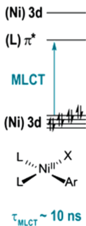
Figure 1.2: Electronic structure of d^8 \text{Ni}^{\text{II}} square planar complexes. Adapted from [23]
