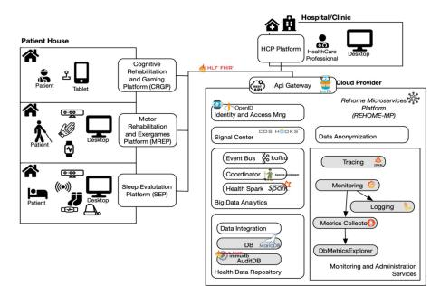
Figure 1. REHOME system architecture.
