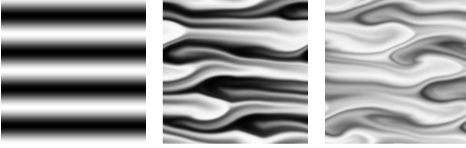
Figure 5.9: Vertical section in the x-z plane at fixed y = 0 of the scalar field \theta for the 3D simulation with \eta = 8 at different times. From left to right: t = 0 , t = 32T_0 , t = 64T_0 .
