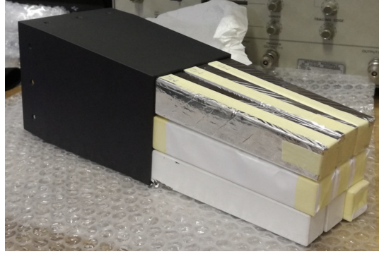
Figure 4.17: The 3D-printed module holder with 9 assembled crystals.
