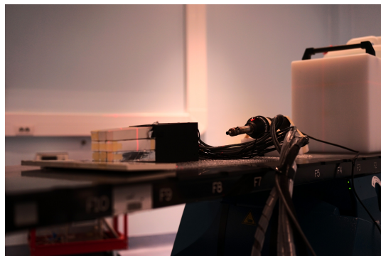
Figure 5.5: Picture of the test beam at CNAO. One calorimeter module laid on the treatment bed with behind the heat gun to simulate temperature changings.
