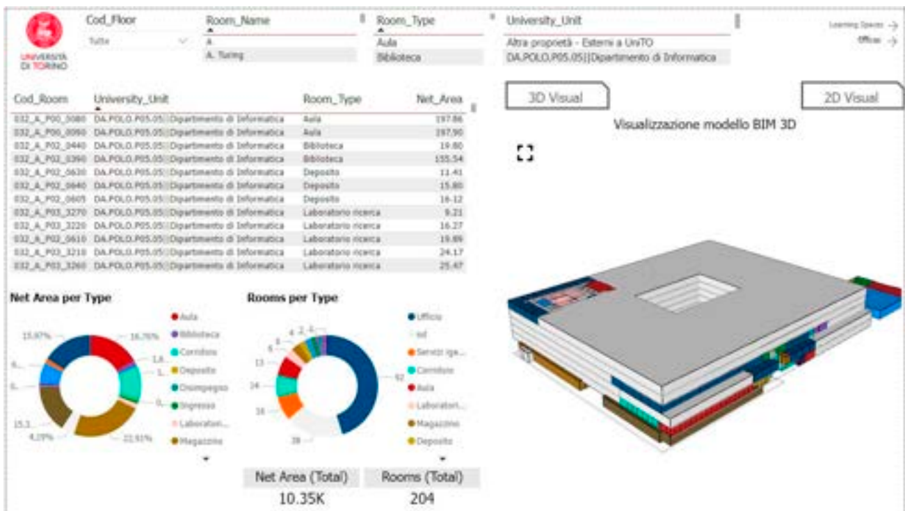
Figure 10. “032_A-B-C_Spaces” dashboard. This represents the Piero della Francesca Center building, giving detailed information about its spaces. Even in this case, a color was assigned to each space’s category for its representation both on the charts and in the model.
