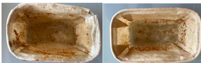
FIGURE 66 APPLICATIVE TEST IN THE OVEN OF A MOLD MADE OF GRASS PAPER (LEFT) VS. SILICONIZED PAPER (RIGHT).
