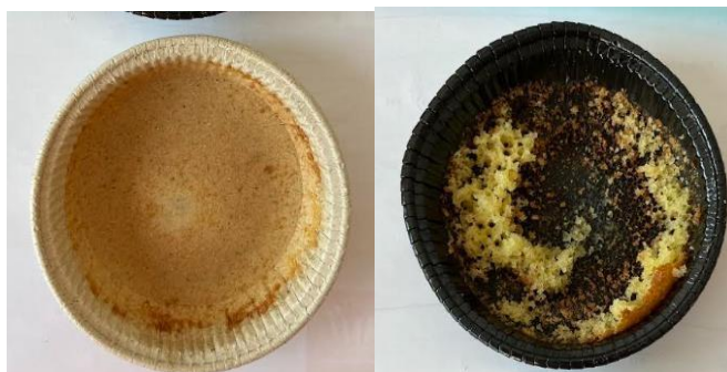
FIGURE 65 APPLICATIVE TESTS WITH BAKED CAKE BATTER COMPARING THE GRASS PAPER SAMPLE WITH SAMPLES WITH PET BARRIER FILM.
