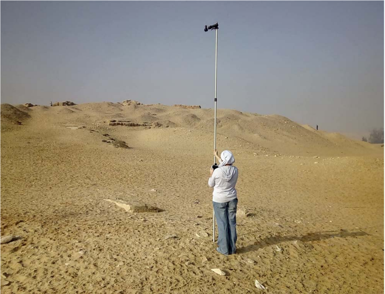
Fig. 4 - Survey of the sun temple causeway by means of Osmo Dji device and tablet mounted on telescopic pole (photo acquisition: A. D'Andrea; elaboration: A. Bosco)
