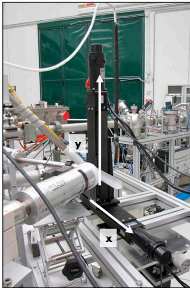
Figure 2. Scanning system at the end of the PIXE beamline.
