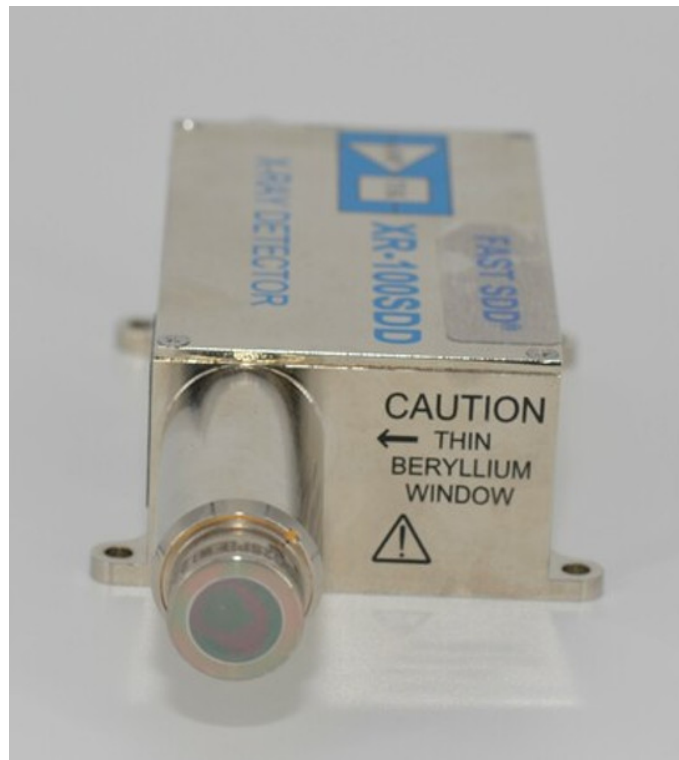
Figure 2.4. Picture of the XR-100 FAST SDD by Amptek.
