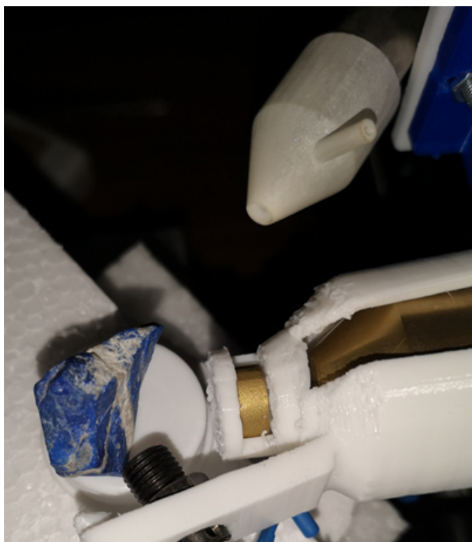
Figure 4.11. Picture of the set-up for the XRIL measurement of the Chilean sample presented in section 2.4.
