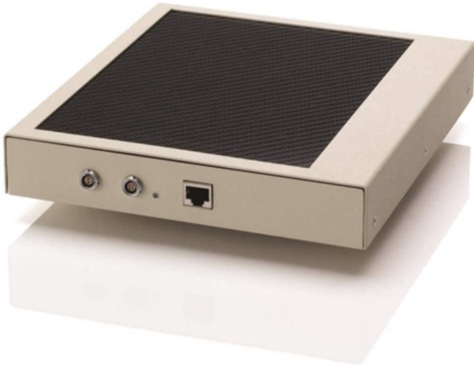
Figure 2.18. Picture of the Shad-o-Box HS detector by Teledyne [72].
