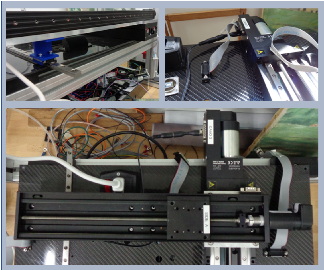
Figure 3.2. Pictures of the top panel of the instrument during its construction. Different positions of the stage of the M404.8PD motor (top left and down), and its connection with a ribbon cable (top right).
