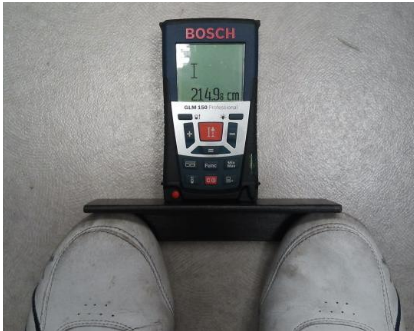
Fig. 22 – Position of the distometer and the L-shaped iron against the feet of the operator
