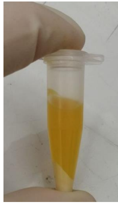
Figure 18. Top and bottom phases after centrifugation of NLCs suspension.
