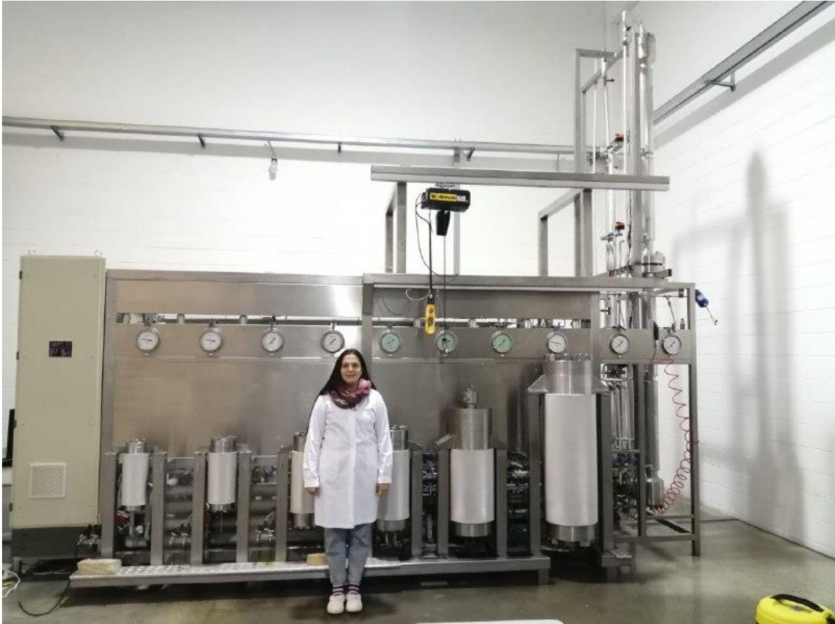
Figure 4. The Exenia plant used for extraction with supercritical carbon dioxide.
