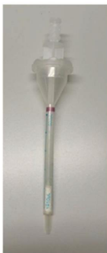
Figure 4. Eppendorf syringe packed with CYPHOS
