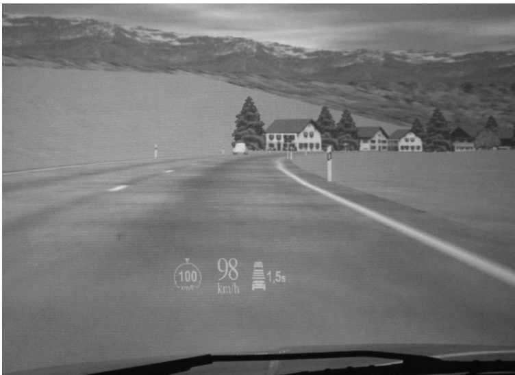
FIGURE 3. The driver's view of the head-up display. The desired speed is on the left, the desired headway is on the right and the current speed is in the centre.
