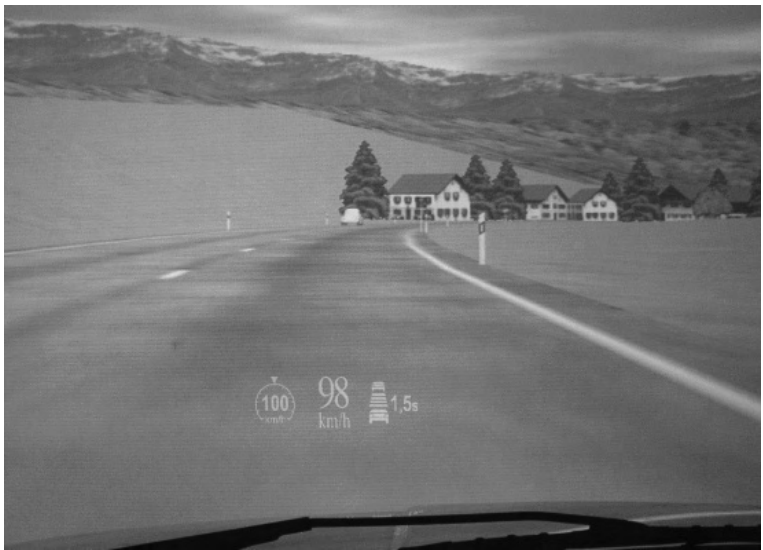
FIGURE 3. The driver's view of the head-up display. The desired speed is on the left, the desired headway is on the right and the current speed is in the centre.
