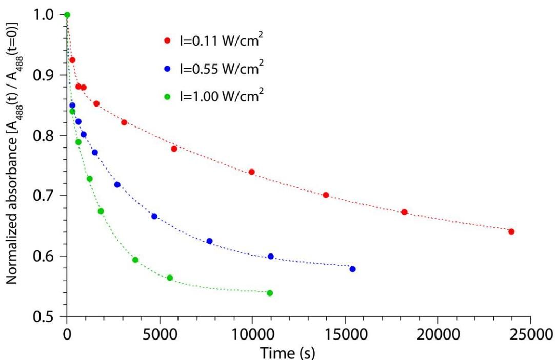
**Figure 5.** Plots of absorbance at 488 nm vs time for a PBS solution of  $1[\text{ClO}_4]_2$  irradiated at three different illumination intensities (488 nm). Dotted curves are the fits to experimental data by means of eq. S4.8 (Supporting Information).
