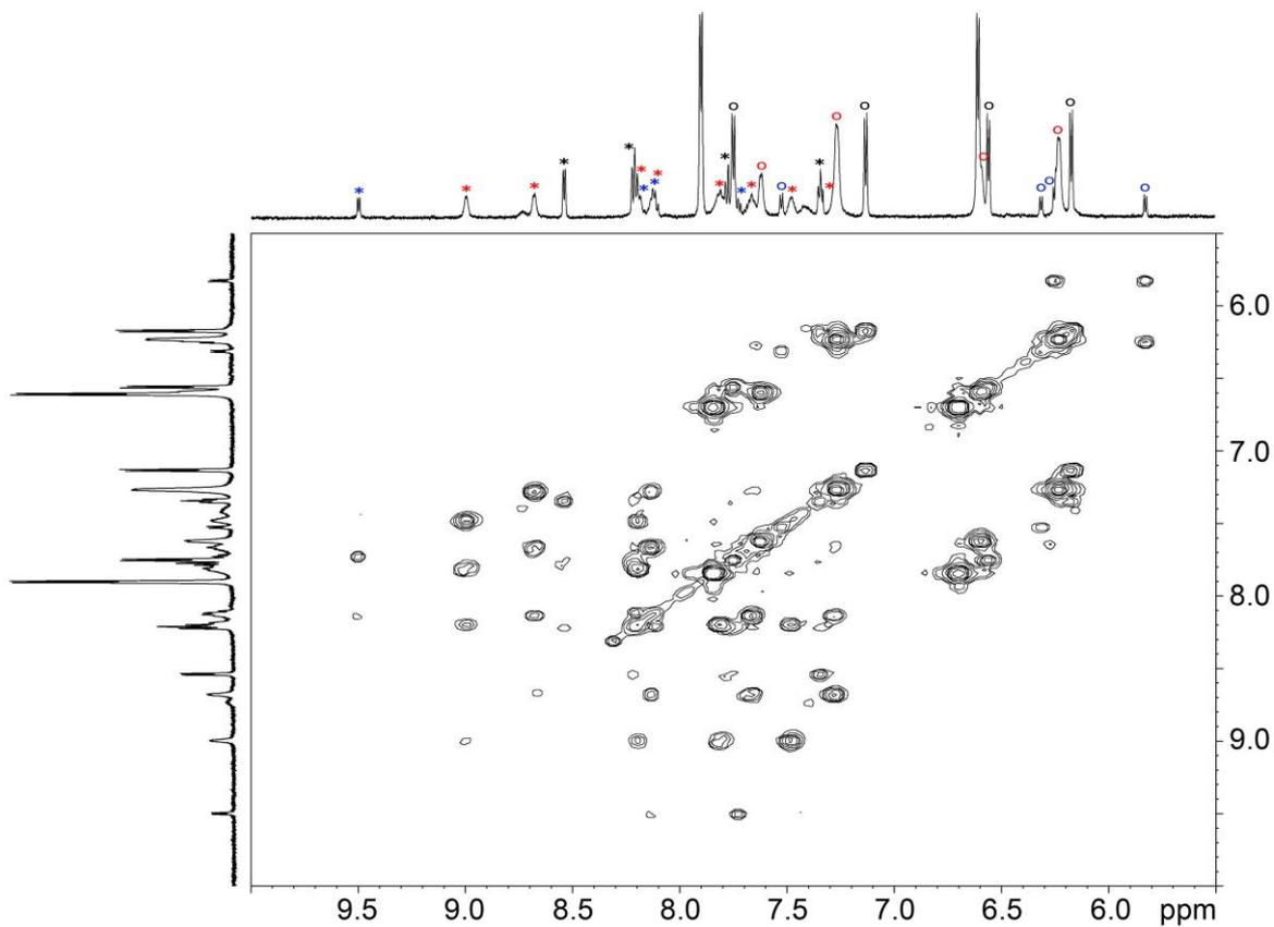
**Figure 7.** 2D  $^1\text{H}$ -TOCSY NMR spectrum of **1** in NaCl 22 mM in  $\text{D}_2\text{O}$ . In 1D  $^1\text{H}$  NMR spectrum peaks were assigned as follows: **1** (bpy \*, 4APs o); **2a** (bpy \*, 4APs o); **3a** (bpy \*, 4APs o).
