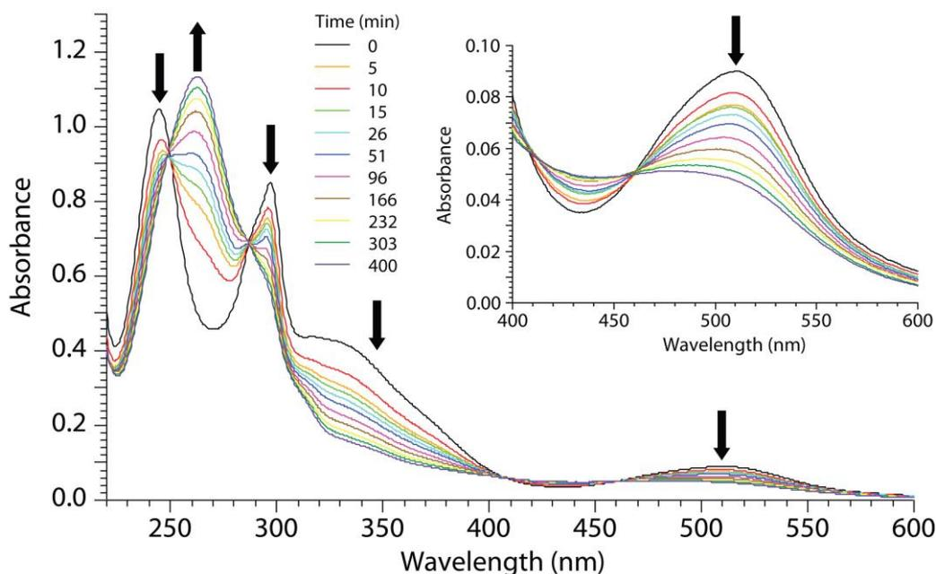
**Figure 4.** Absorption spectra of  $1[\text{ClO}_4]_2$  in PBS solution irradiated by a 488 nm  $0.1 \text{ kW/cm}^2$  laser beam for different times (see legend). Inset: enlargement of the 400-650 nm region.
