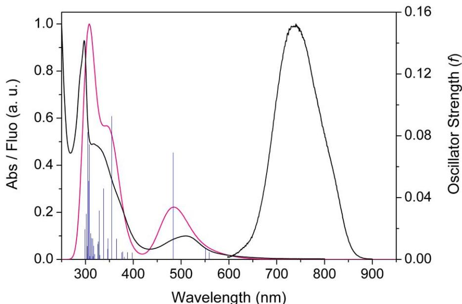
**Figure 2.** Calculated (magenta line) and experimental (black line) absorption and emission (black line) spectra of **1** in  $\text{H}_2\text{O}$ . The excited states are shown as vertical bars with heights equal to the oscillator strength values. The theoretical curve was obtained using the program *GussSum 1.05*.
