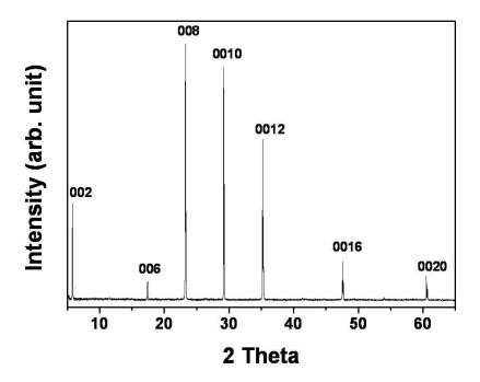
Figure 2: XRPD pattern for the sample synthesized at 864°C growth temperature ( $\delta$  batch) obtained in asgrown conditions. Background signal has been subtracted.
