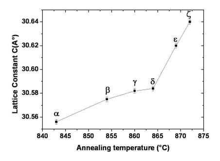
Figure 3: c-axis lattice constant for Bi-2212 whiskers versus the synthesis growth temperature (Greek letters refer to the synthesis batches reported in table 1).
