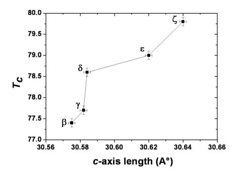
Figure 4: Plot of the  $T_c$  values vs the c-axis lattice parameters of the whiskers collected from the different synthesis batches. Greek letters are the synthesis identifier as reported in table 1. Error bars for both the  $T_c$  and c-axis values are reported.
